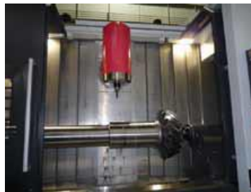
Figure 8 - Pinion workpiece on multitasking machine
